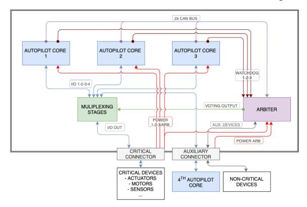
This hardware has been designed so there is **no single point of failure**. Even in the event of an arbiter failure, the system will automatically assign control to one of the autopilot cores. Redundant configuration includes redundant power input so multiple batteries can be used for powering the system.
